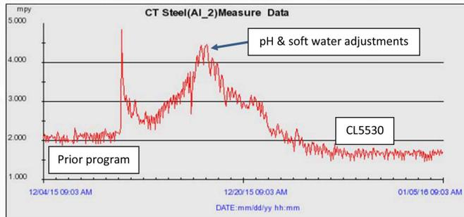
As shown on the graph to left, once all of the system chemistries were set, corrosion rates eventually decreased from 2.1 to 1.6 mpy. Corrosion coupons are also being used to monitor program performance and have correlated very well with the on-line corratel readings.
