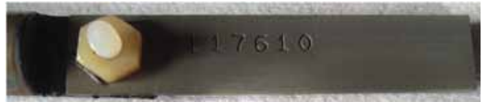
Figure 13. Passivated steel coupon after 2 day exposure to pH 3 cleaning solution containing RPC
