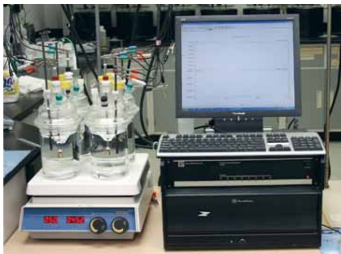
Figure 1. Potentiostat arrangement used for electrochemical studies
