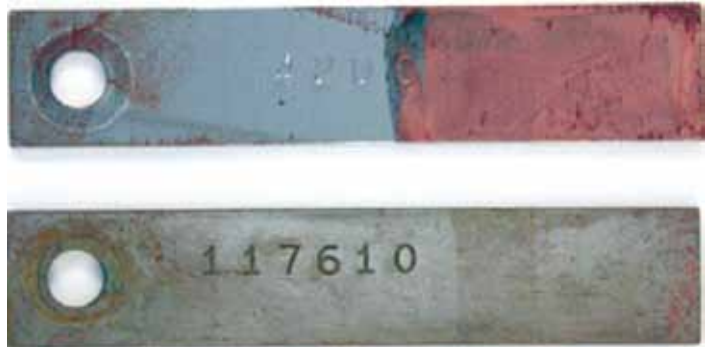
Figure 15. New coupon (top) and coupon passivated with RPC during the acidic chemical cleaning (bottom) after half-exposure to a 15% copper sulfate solution for 20 seconds. Note the copper plating on the new coupon as compared to the absence of copper plating on the RPC-passivated coupon.
