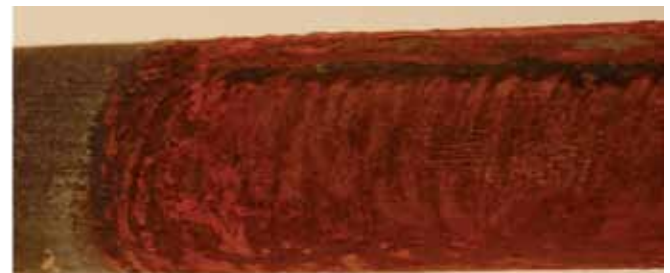
Figure 10. Tube section cleaned with organic phosphate and reducing agent after 24-hour exposure to untreated blank water.
