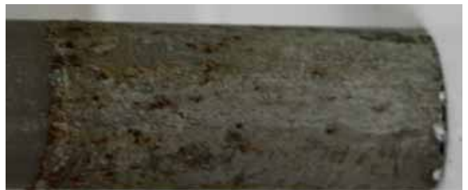
Figure 9. Tube section cleaned and passivated with RPC, organic phosphate, and reducing agent after 24-hour exposure to untreated blank water.
