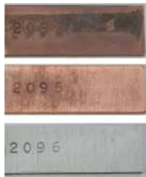
Figure 12. Passivated coupons after 20 sec. exposure to 15% CuSO 4 solution
