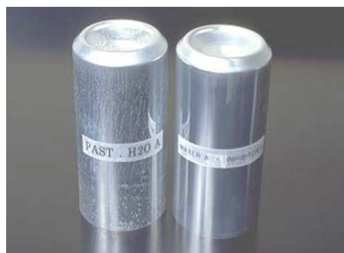
Figure 2: The can on the left shows the deposition of calcium salts and other organic contaminants, which create the appearance of spots.
